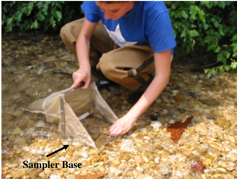
Figure 1. Sampling using the quantitative Surber Sampler. (Photo courtesy of Emily Duncan)
