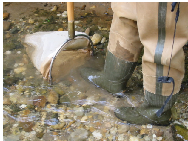
Figure 2. Sampling using the D-net. (Photo courtesy of Emily Duncan)
